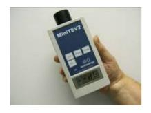
The MiniTEV2 is used to detect and measure TEV activity. The magnitude and rate of the TEV discharge activity is displayed on a LCD screen. A simple calculation is used to determine the severity of any discharge found.
