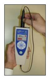
Disconnect the function checker after checking the UltraTEV Plus+; do not attempt to use the UltraTEV Plus+ with the checker plugged in.
